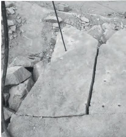
extraction of large blocks by complex gap blasting
