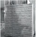
grooves come from the individual holes for the explosive charges). After the first cut the barrel height and the lid are cut out of the rough stone with a diamond wire saw. (image 1)
