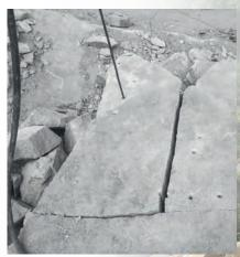
extraction of large blocks by complex gap blasting
